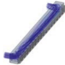
An additional linear CeramCool® version is designed to cool high-power LEDs. Depending on the requirements Rubalit® or Alunit® may be used for the same geometries. On a length of 120mm this makes it possible to cool 290W or 640W, respectively.
