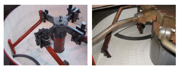
ALOTEC ceramic linings have proven to be effective for virtually all makes and types of agitator. The high wear resistance of the material ensures long life and increased efficiency.
