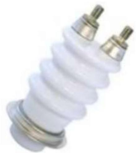
On some terminal designs, the cap-stud or cap-lug assembly is integrated with a conductor passing through the hollow inside of the body. This conductor is used for the internal connection in the apparatus. On other designs, this internal conductor is inserted by the customer and joined with the cap upon installation of the terminal. Terminal mounting flanges of Ceramaseal® terminals are joined to the apparatus housing by various welding, brazing, and soft soldering techniques.
