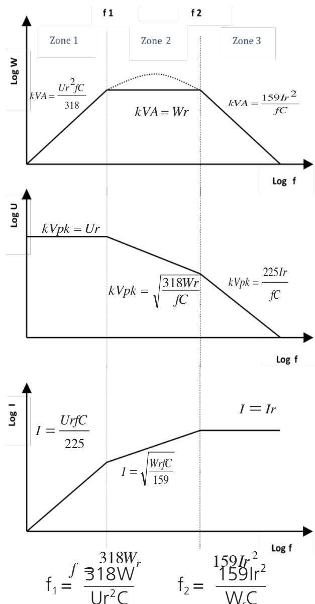
At frequencies below  $f_1$  (Zone1) the capacitor can be operated at its maximum ac rating  $U_r$ .
